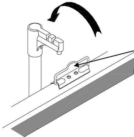
When attaching/detaching the screen to the pull hook, please be sure to raise the screen using the handle indicated here as pulling on other parts of the top support bar may cause damage to the screen. Make sure to firmly hold the handle to avoid the screens from suddenly retracting into the housing.
